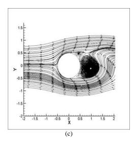
Figure 3:- Streams lines at Re = 200 for (a)  $\alpha = 0^0$ , (b)  $\alpha = 5^0$ , (c)  $\alpha = 10^0$
