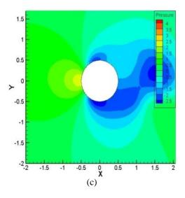
Figure 8:- Pressure contours at Re = 1000 for (a)  $\alpha$ = 00, (b)  $\alpha$ = 50, (c)  $\alpha$ = 100
