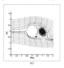
Figure 4:- Streams lines at Re = 500 for (a)  $\alpha$ = 0 $^{0}$ , (b)  $\alpha$ = 5 $^{0}$ , (c)  $\alpha$ = 10 $^{0}$
