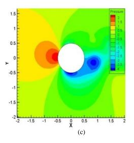
Figure 6:- Pressure contours at Re = 200 for (a)  $\alpha$ = 0°, (b)  $\alpha$ = 5°, (c)  $\alpha$ = 10°
