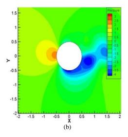
Figure 7:- Pressure contours at Re = 500 for (a)  $\alpha = 0^0$ , (b)  $\alpha = 5^0$ , (c)  $\alpha = 10^0$
