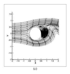
Figure 5:- Streams lines at Re = 1000 for (a)  $\alpha$ = 0°, (b)  $\alpha$ = 5°, (c)  $\alpha$ = 10°
